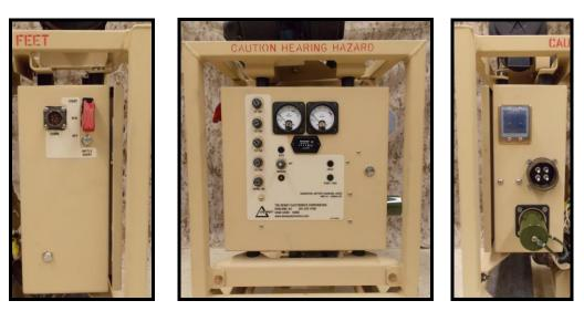
A simplified control box allows the generator to be placed in auto mode with the flip of a switch. Output voltage and loads are monitored on the analog meters. An engine hour meter is located on the front panel along with LEDs that provide status and fault indications. A digital data connector and battle short switch are located on one side panel and the main circuit breaker. A NATO slave for electric starting and a generator output connector to loads are located on the other side panel.
